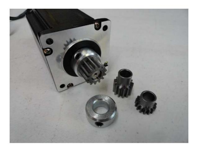
The gears are designed to lock onto the 3/8" shaft of the 620in-oz motors supplied by candonc. The procedure follows:
