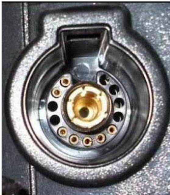
**2: Dissassemble the plug of the hand torch and install an additional pin to make the connection.**
