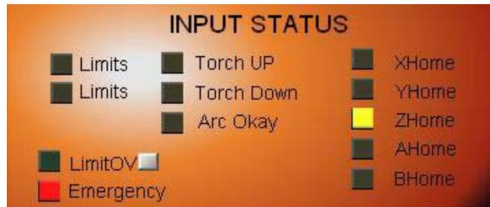
Go to the diagnostics page of Mach 3 and you will see the INPUT STATUS in the upper right hand corner. Lift the torch to trigger the switch and the indicator next to the ZHOME should turn yellow.
